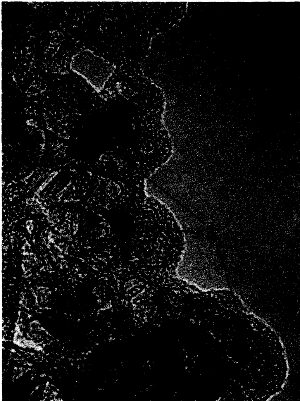
FIG. 7. (a) and (b) High-resolution images of Pt on graphitized channel black.
