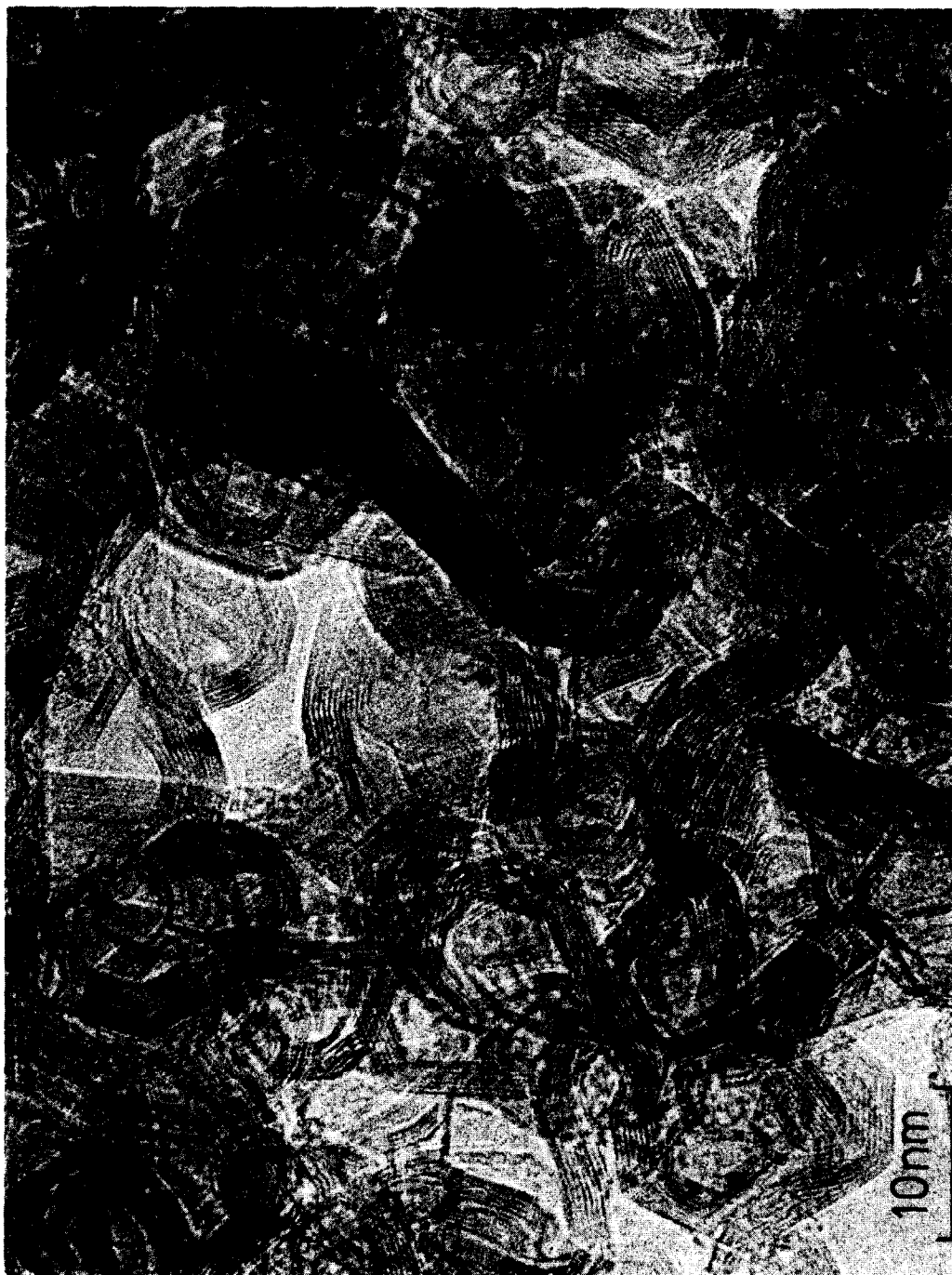
FIG. 2. High-resolution image of Pt on graphitized channel black.
